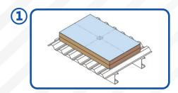
Mark the installation position of Anchor base on the roof
