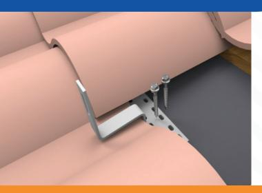
Our Chiko Solar S-Tile Kit is made of SUS304 Stainless Steel. It is designed for use on curved S-Tile roofs. Our hook is installed under the existing roof by removing a tile and placing it back in its original place after the hook is secured to the underlying rafter. It does not require modification to the structure, maintaining the structure's integrity. Chiko guarantees a quick, easy installation with long lasting quality. Please follow the installation manual for proper installation
